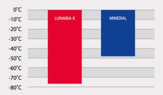
Comparative Floc Point of LUNARIA K and Mineral Oils Results shown above indicate the temperature at which wax in the oil precipitates in refrigerant / oil mixtures lead to clogging
