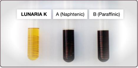
Results shown above were obtained through ageing the oil at 110°C for 96 hours under an oxygen flow rate of 1L/hr in the presence of a copper catalyst
